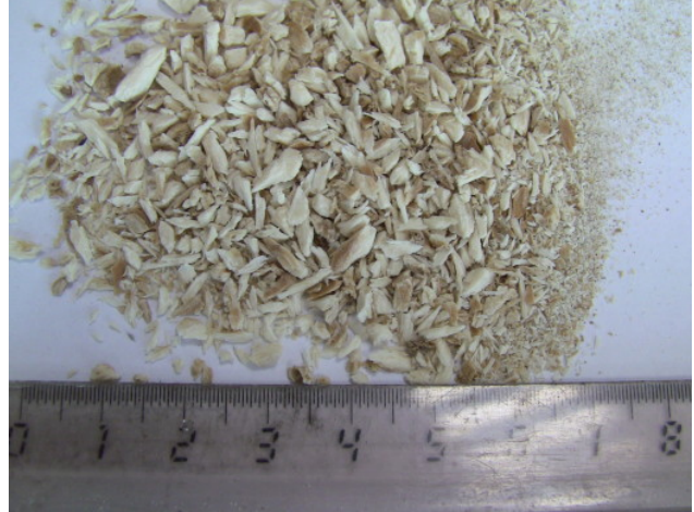
Picture 6: Sample 3 after pre-cutting in SM 200
