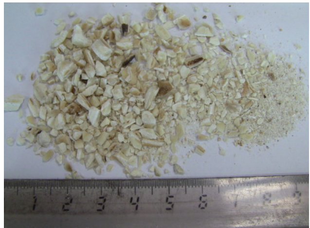
Picture 4: Sample 2 after pre-cutting in SM 200
