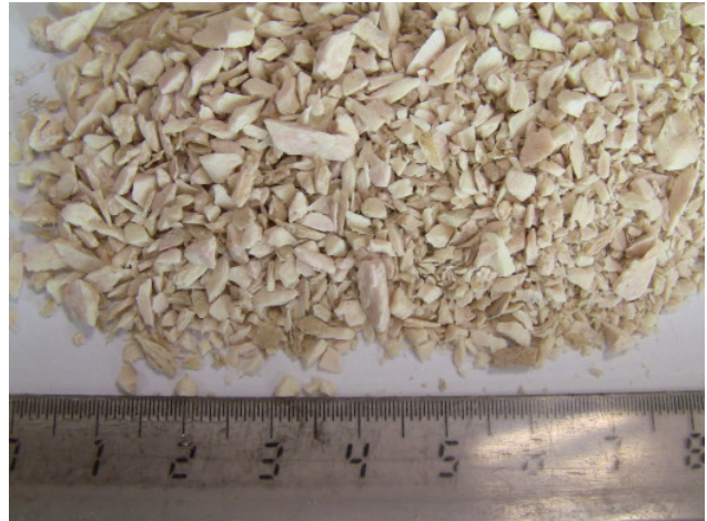
Picture 2: Sample 1 after pre-cutting in SM 200
