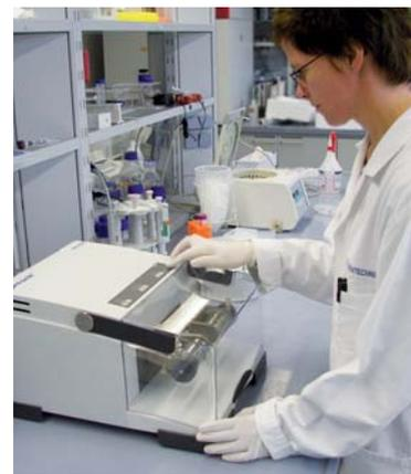
Gisela Boehle uses the Retsch Mixer Mill MM 400 to grind wool samples
