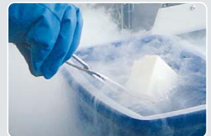
Embrittlement of the sample in a stainless steel grinding jar with liquid nitrogen
