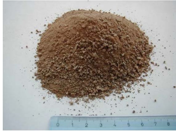
Fig. 2: After crushing in BB 51 with gap size of 1.0 mm
