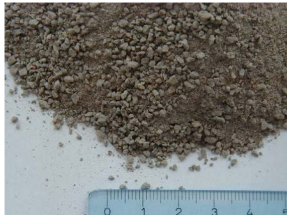
Fig. 4: After crushing in BB 51 with gap size of 1.0 mm
